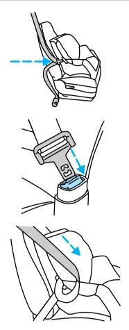
7. Pull the lap belt portion across the child seat toward the buckle and pull up on the shoulder belt while pushing down with your knee on the child seat.
